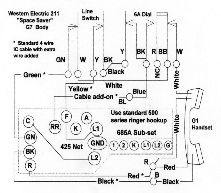
N.B. - If 211 is equipped with F-1 handset, disregard the 2nd white receiver conductor connected to terminal "R". That connection has already been established inside the F-1 handset itself.
